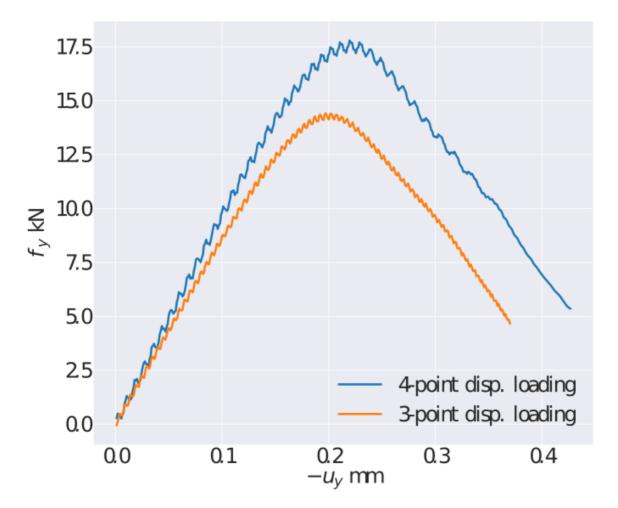
Here we plot the deflection of point at the center (0.8, 0.125) of the beam. The force is the total force experienced by mesh node at  $P_{load}$  in case of 3-point test and sum of total force experienced by mesh node  $P_{load,1}$  and  $P_{load,2}$  in case of 4-point test. We believe the small oscillations seen in the plot are due to the dynamic nature of simulation.
