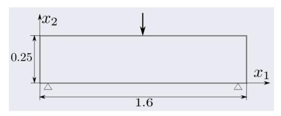
Four point test. Displacement  $u_2(t) = -t\gamma$  is specified at point  $P_{load,1} = (0.6, 0.25)$  and  $P_{load,2} = (1.0, 0.25)$ .
