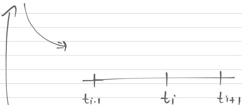
$$\frac{dy}{dt}(t_i) \approx \frac{y(t_i) - y(t_{i-1})}{\Delta t_{i-1}}$$
