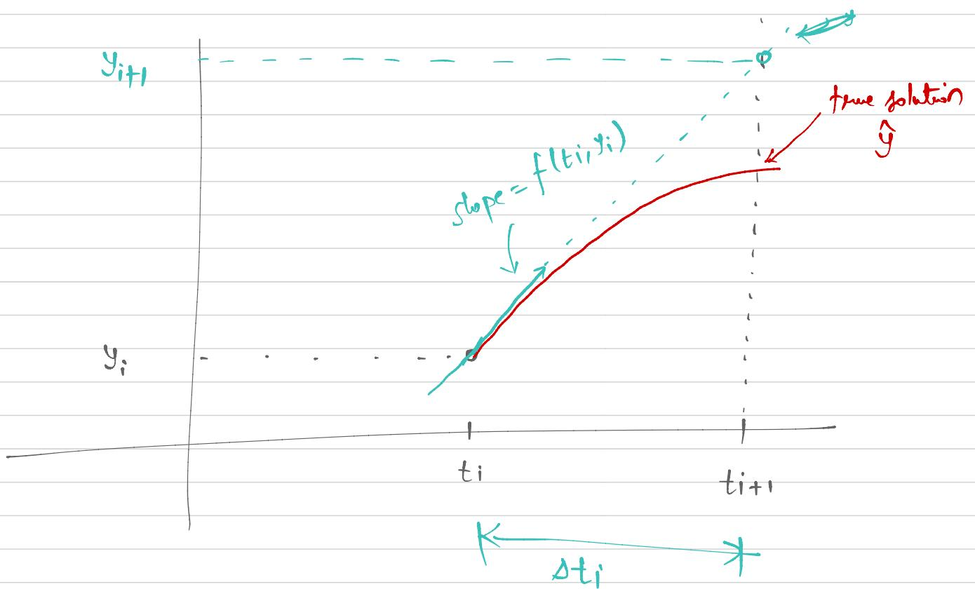
$(t_i, y_i)$  &  $(t_{i+1}, y_{i+1})$  are on straight line
