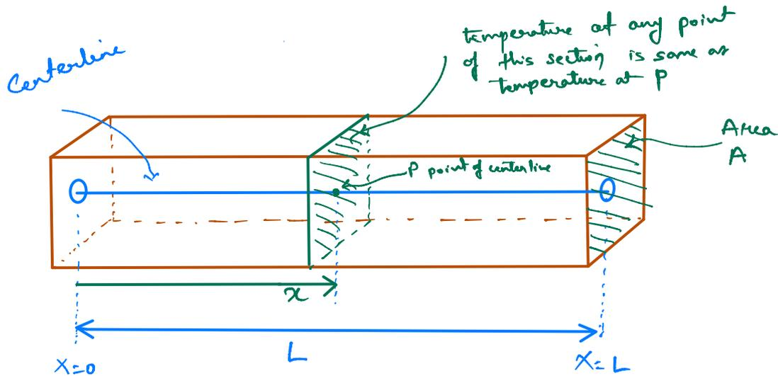
Figure 1: Thermal heating of the bar with a uniform cross-section.
